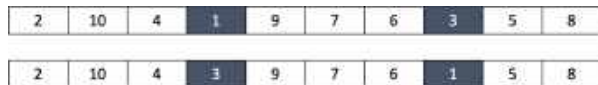
Fig. 6. 2-opt example, the first array contains a permutation from 1 to 10, it was chosen two items to interchange it into the second array
