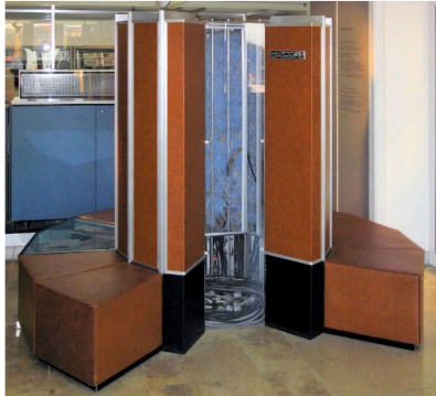
The Cray-1 Supercomputer was the first to really take advantage of the liquid cooling that we think of today.
