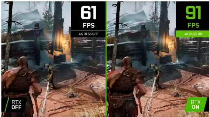
Super sampling uses machine learning to improve frame-rates by effectively predicting what the frame should look like through pattern recognition.
